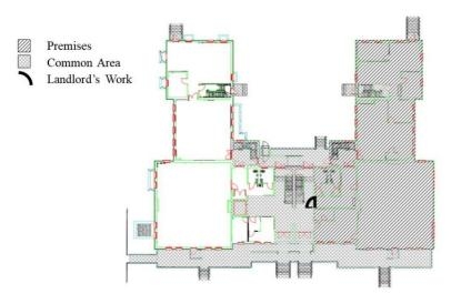
Includes framing and installing an aluminum and glass storefront door at the entrance to the suite as depicted. The door will have a lock that is badge accessible similar to the front door of the building. Includes creating a demising wall on the back stairwell to separate the second and first floors as is depicted. All work will be done per code, i.e., fire/life safety systems and signage addressed. Includes moving the Post Office box to a spot in the common area lobby.
